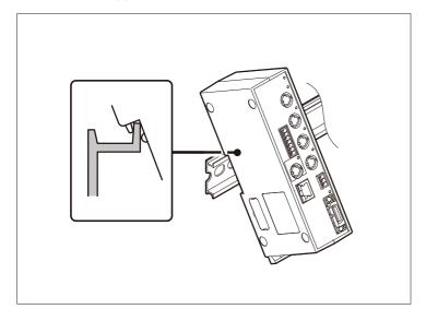
2. Push and install the MG41 main unit until a click is heard so that the lower side of groove on the back of the MG41 main unit is fit into the DIN rail.
