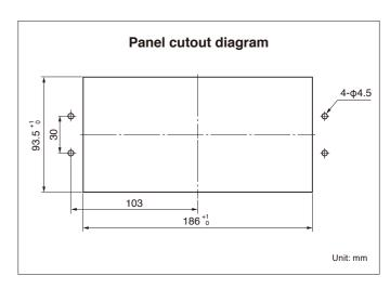
Reference: If a mounting screw hole cannot be drilled in the panel, the MG43 may be installed using four screws on the back of the main unit.
