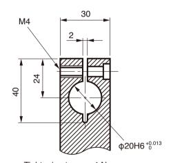
Tightening torque: 4 N·m Hex. socket head bolt M4 is used.
