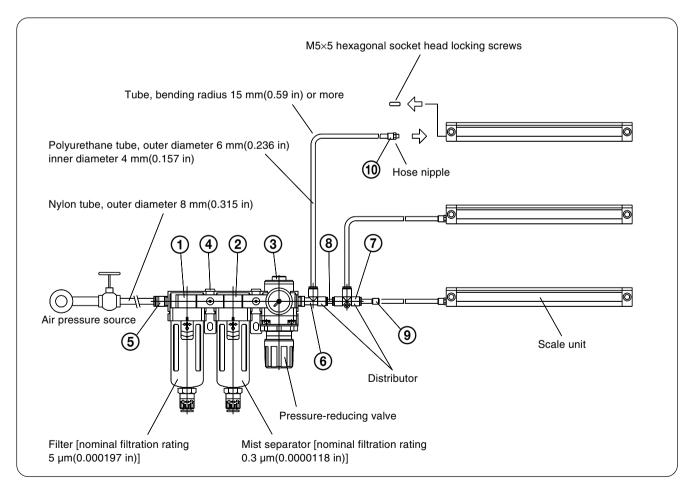
• The air supply unit and fittings should be provided by the customer. The tables below provide standard equipment specifications and component parts (manufacturers) for reference.
