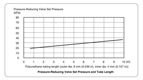
This diagram shows the relationship between the set pressure for the pressurereducing valve and the tube length for an intake air pressure of 20 kPa.
