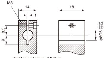
Tightening torque: 0.6 N⋅m Material: In case of SUS303
