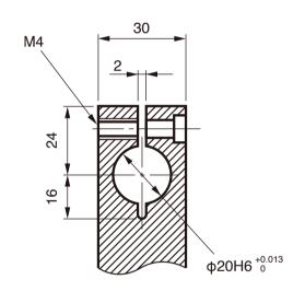
Tightening torque: 4 N·m
